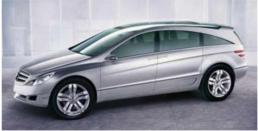
The GST design displayed in Detroit was a six-passenger, 15-foot-long vehicle with a 5.5-liter V8 engine. The concept has 22-inch tires, butterfly side doors that open 90 degrees in opposite directions, and a glass roof that tints at the touch of a button.
